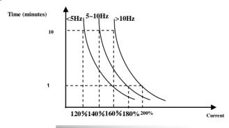
Fig 6-21 Motor overload protection value
