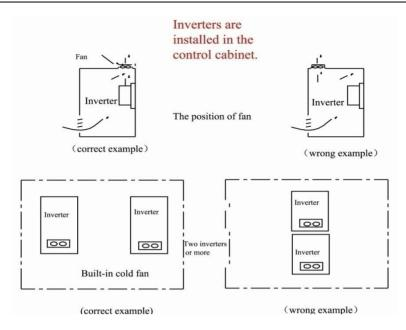
Fig 1-2 Installed in the cabinet
