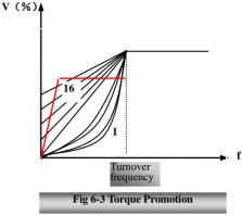
If the torque is elevated too much, motor is easy to overheat, and the current of inverter will be too high. Please check the motor while elevating the torque.
