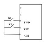
Two-line mode 2: when this mode is used, FWD is enable terminal, the direction is controlled by REV terminal.
