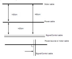
Generally, the control cables should be shielded cables and the shielding metal net must be connected to the metal enclosure of the drive by cable clamps.
