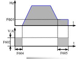
Figure 5-18 DC braking
