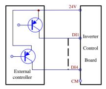
Wiring by source electrode is a mode most in use at present. Wiring for control terminal is connected by source electrode, user should choose wiring mode according to requirement.
