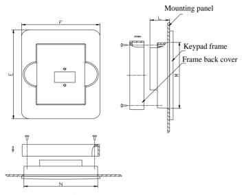
Fig.3-6 Panel mounting structure
