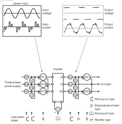
**Examples of Measuring Points and Instruments**
