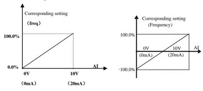
Fig 6-14 correspondence of analog input to setting
