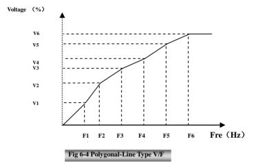
Note: during the process of speed track, polygonal-line V/F curve function is invalid. After speed track is finished, this function is valid.
