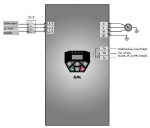
Figure 5-1 Wiring Diagram
