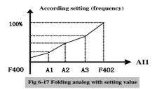
F400 and F402 are lower/upper limit of analog AI1 input. When F460=1, F462=2.00V, F463=1.4, F111=50, F203=1, F207=0, then A1 point corresponding frequency is (F463-1) \*F111=20Hz, which means 2.00V corresponding to 20Hz. The other points can be set by the same way.
