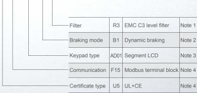
Note 1: R3: EMC C3 level, test condition: power cable is 25m shielded wire.
