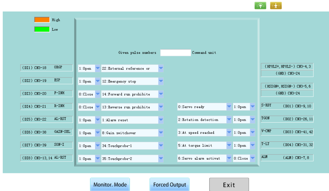
Fig 3-2-13 IO Terminal Configuration Interface
