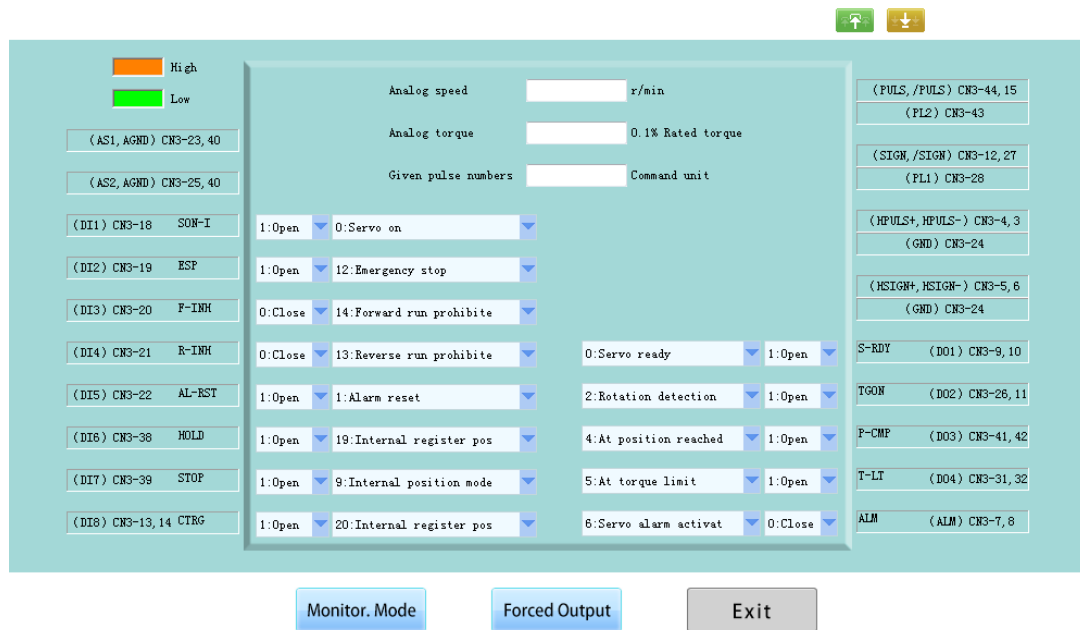
Fig 3-1-16 IO Terminal Configuration Interface
